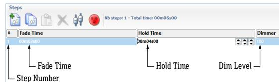
12. Create additional steps as needed by repeating steps 9 - 11. Play your scene and make adjustments to the parameters as desired. When a scene is complete, save as a Show File (.dlm) as a backup on your computer. Create up to 24 scenes using the Editor tab.
