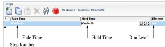
12. Create additional steps as needed by repeating steps 9 - 11. Play your scene and make adjustments to the parameters as desired. When a scene is complete, save as a Show File (.dlm) as a backup on your computer. Create up to 24 scenes using the Editor tab.
