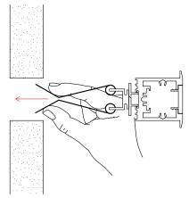
**5.** Release spring-loaded arms, allowing the spring tension to pull fixtures into place.
