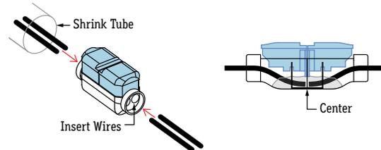
3. Use pliers to push splice buttons down until they sever the wire and snap into place.
