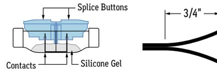
2. Push wires into connector until they stop at the center point. Repeat process for other side.
